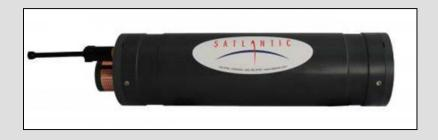
The SeaFET sensor measures pH with an ion-sensitive field effect transistor (ISFET). The advantages of the ISFET include robustness, stability, and precision that make it suitable for ocean pH measurement at low pressure.
